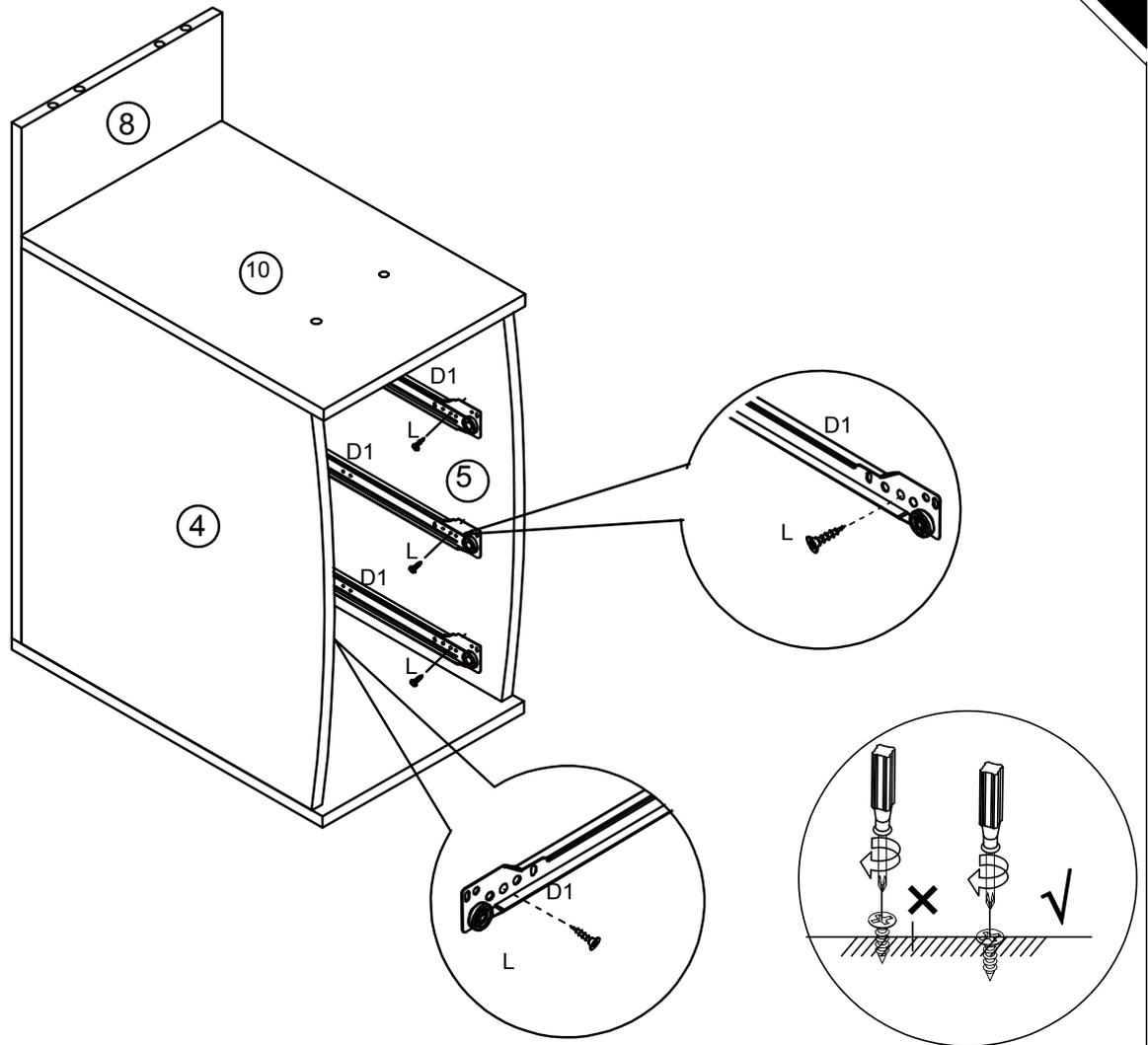
**EN** Please find the exact hole for installation, otherwise it will be misaligned. The screws on the drawer slide must be leveled, otherwise it will affect the smoothness of the drawer.
