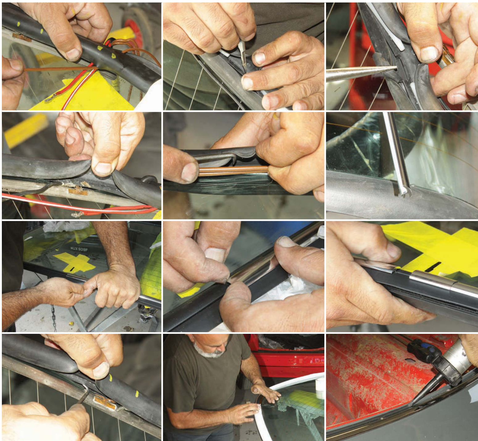
Sliding the wires into position inside the new rubber is only half of the job – on older cars in particular you will probably have to make some repairs to the connections. Then you need to add the trim strips – without the rubber falling off the edge of the window, of course. Easier said than done, but having all components spotlessly clean and grease-free helps. Tape (bottom row, middle) should prevent rubber becoming dislodged while window is fitted to the car. Rubber designed to sit on a small bead of sealant
