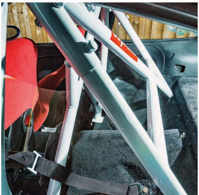
Bolt-in rear cage has been refinished in white, while Recaro Pole Position seats are trimmed in red, the work of Capital Seating in Leicester
