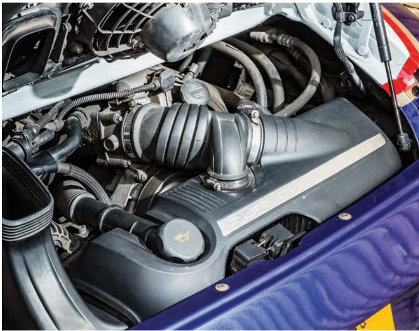
Engine is largely stock, aside from the exhaust system. Front luggage bay is now dominated by the reservoir required by the Air Lift suspension system
