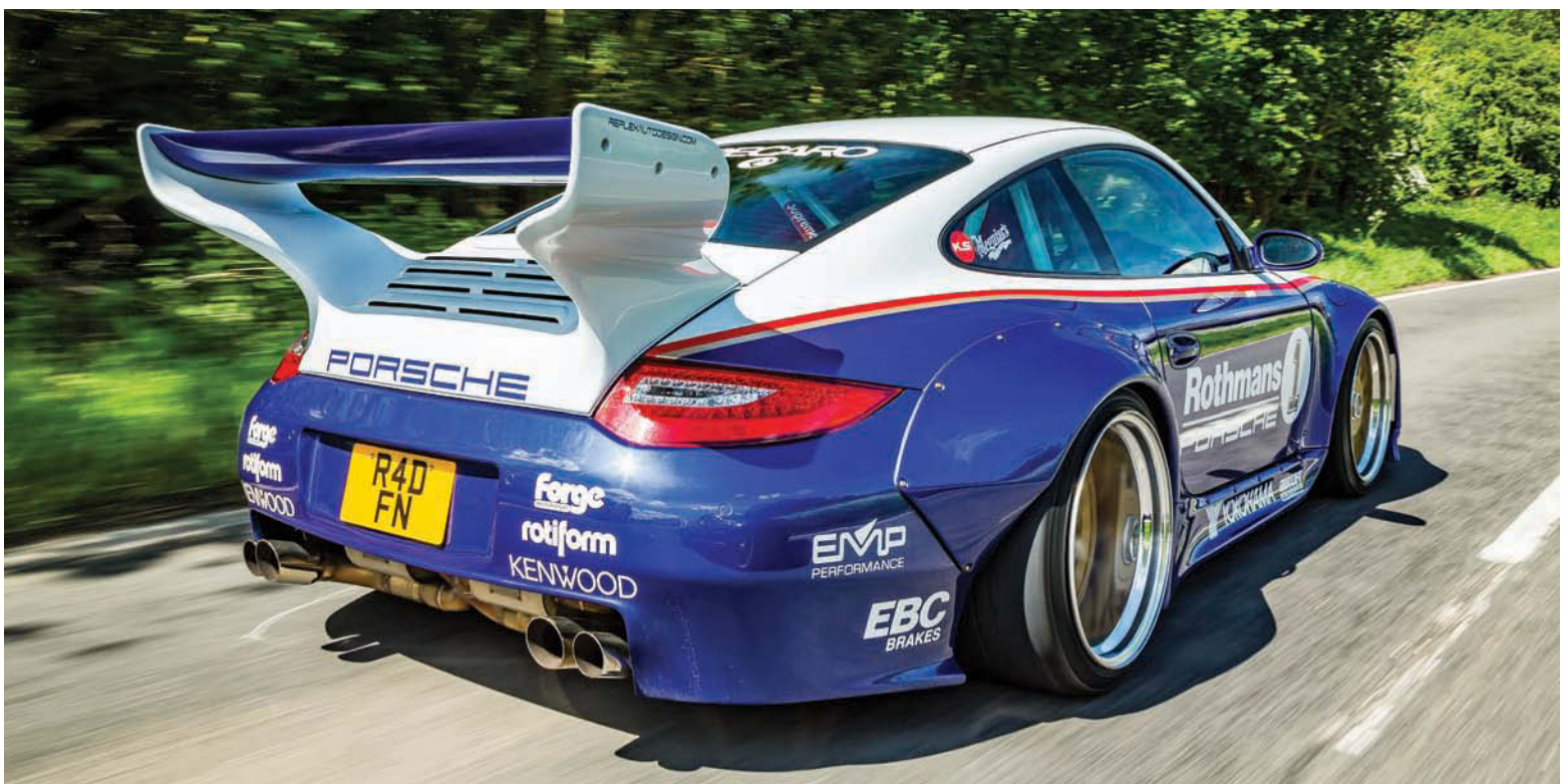
Rear apron has been remodelled to expose the custom-built EMP exhaust system. Beautifully finished, it emits a purposeful roar without causing an annoying drone cruising at speed
