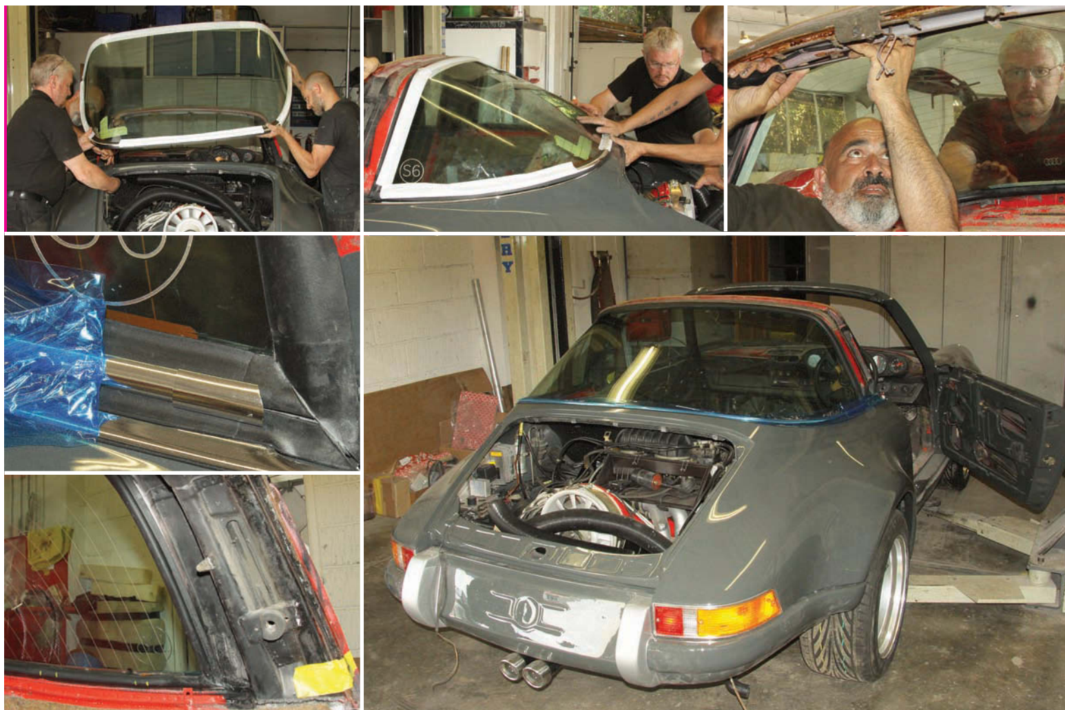
It's a three- and occasionally even a four-man job to hold the assembled screen in the correct position, while someone inside the cabin eases the lip of the rubber over the small but none the less awkward flange on the body. In the Porsche factory they probably used the old-fashioned string method, but Paul Ralhan prefers to use an angled pick. Either way, take great care not to tear the rubber. Main picture shows screen safely in position, but still to be secured by the stainless-steel cover for the roll-over hoop
