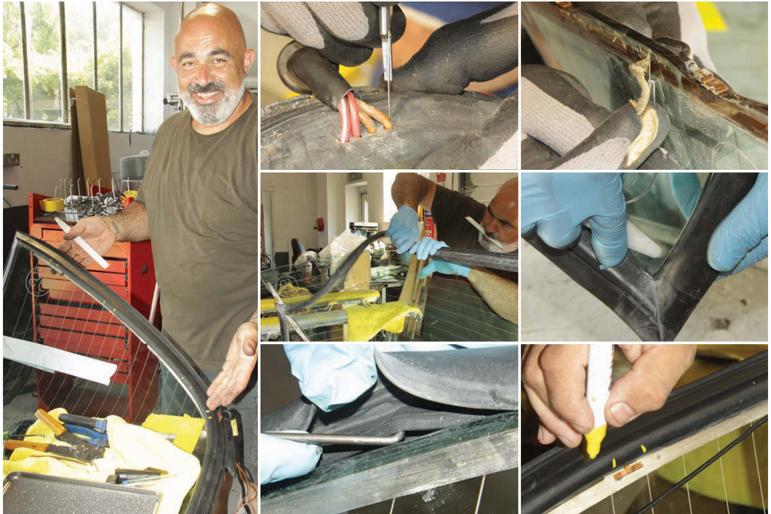
One of the first stages in the process is to cut the wires for the heated rear window out of the old rubber – although such will likely be the aggravation involved in fitting them to the new extrusion, and then fitting that over the edge of the glass, that you might consider simply abandoning the HRW facility. Paul Ralhan (far left), working on a customer's car, didn't have that option, of course – hence his obvious satisfaction in finally having the assembly ready for installation. And that, too, will be a bit of a battle...
