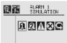
Figure 16. Alarm/Fault Simulation Menu
