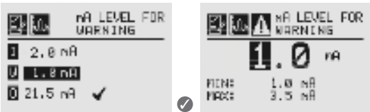
Figure 13. Set mA Levels for Warning
