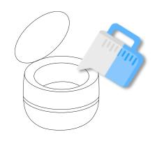
Open the lid and fill the stainless steel tank with water. WARNING: Running a device without water may damage it!
