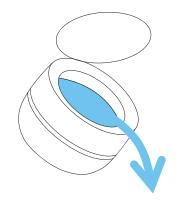
After the cleaning process is finished, unplug the power cord, open the lid, and remove the aligner. Lastly, pour the water out of the tank from the arrow direction. Clean and wipe the tank.
