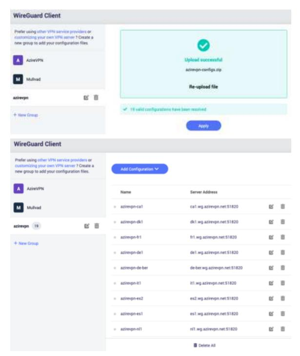
**Manually Add Configuration** is for if you want to paste the WireGuard configuration or fill in each item.
