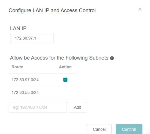
By default, each node can access other's LAN, based on security, we recommend only open the corresponding service IPs.
