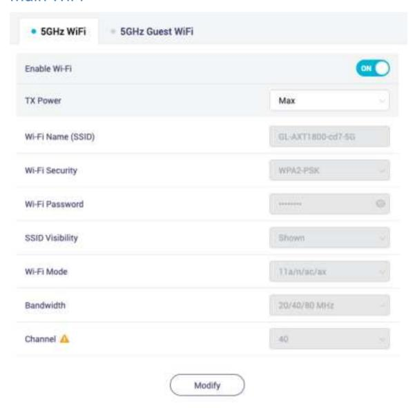
Note: The Channel can't be modified when repeater is enabled.
