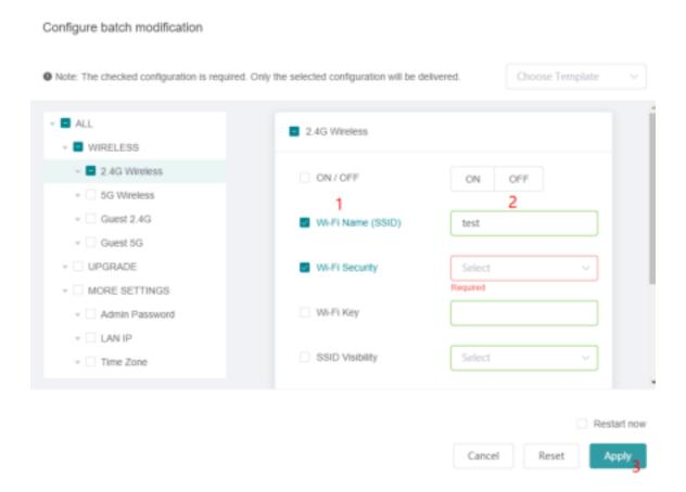
The checked configuration is required, and only the configuration that conforms to the rule can be filled out. After the configuration is delivered, it does not take effect immediately. The configuration takes effect and the device needs to be restarted. You can check the Restart now option in the
