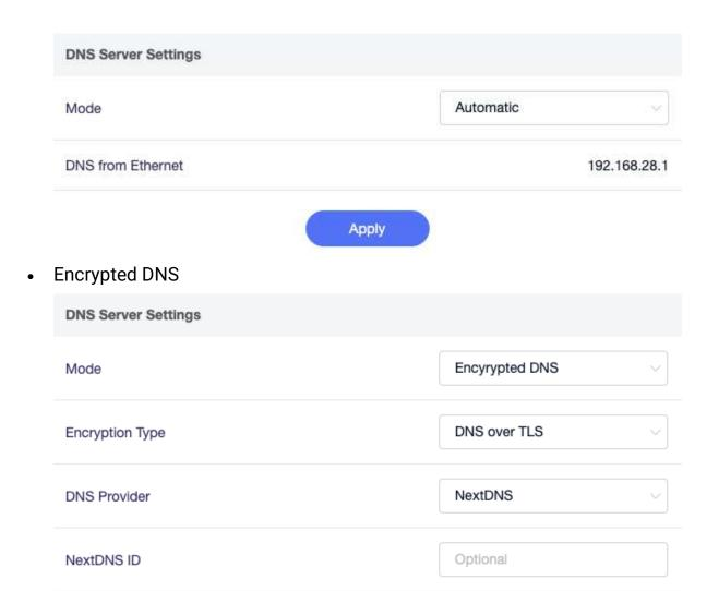
**Encrypted Type** has four type, DNS over TLS, DNSCrypt-Proxy, DNS over HTTPS, Oblivious DNS over HTTPS.
