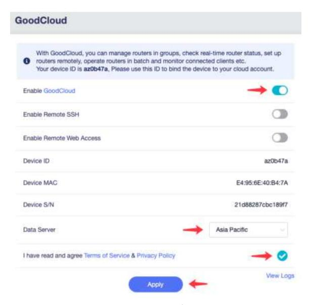
Follow the steps above, to enable the cloud function, which will allow the router to connect to the GoodCloud server.
