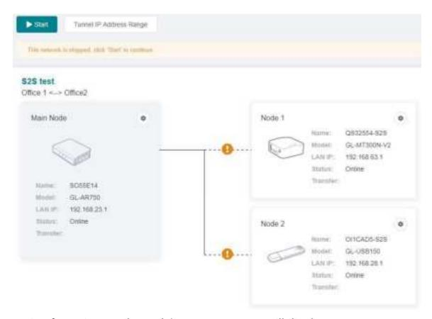
Wait a few minutes, the node's connect status will display as lines. Solid line means connected, dashed line means disconnected.
