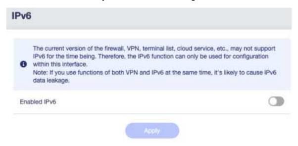
The current version of the firewall, VPN, terminal list, cloud service, etc., may not support IPv6 for the time being. Therefore, the IPv6 function can only be used for configuration within this interface.
