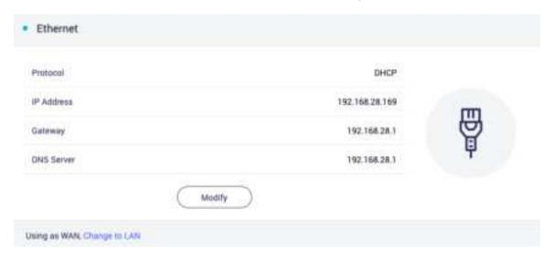
**Note**: Before plugging the Ethernet cable into the WAN port of the router, you can click **Change to LAN** to set the WAN port as a LAN port. That is useful when you are using the router as a repeater. As a result, you can have one more LAN port.
