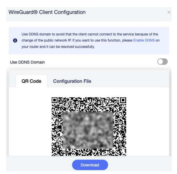
If your network's public IP changes from time to time, you can enable DDNS, then using DDNS domain in the configuration.
