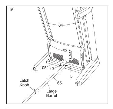
17. Attach the upper end of the Storage Latch (65) to the Frame (64) with a 3/8" x 1 3/4" Bolt (7) and a 3/8" Nut (13).
