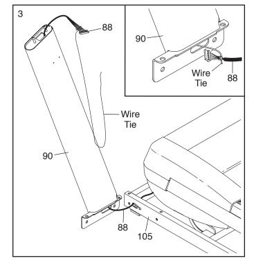
4. Hold the Left Upright (90) against the Base (105). Be careful not to pinch the wires. If necessary, position the base ground wire (A) in the hole in the side of the Left Upright. Insert two 3/8" x 2 3/4" Screws (8) and two 3/8" x 1 1/4" Screws (9) with two 3/8" Star Washers (14) into the Left Upright.
