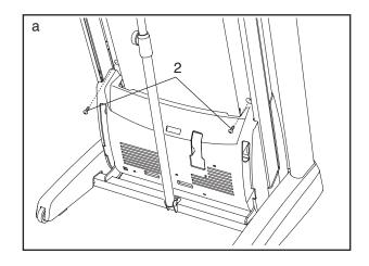
Lower the treadmill (see HOW TO LOWER THE TREADMILL FOR USE on page 29). Remove the three #8 x 3/4" Screws (2). Carefully pivot the Motor Hood (72) off.
