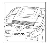
heart rate will be shown. For the most accurate heart rate reading, continue to hold the contacts for about 15 seconds.
