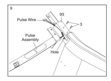
10. Slide the pulse assembly onto the Left and Right Handrails (92, 93). Make sure that the brackets on the pulse assembly are flush against the rubber on the Handrails. Be careful not to pinch the pulse wire against the pulse assembly.
