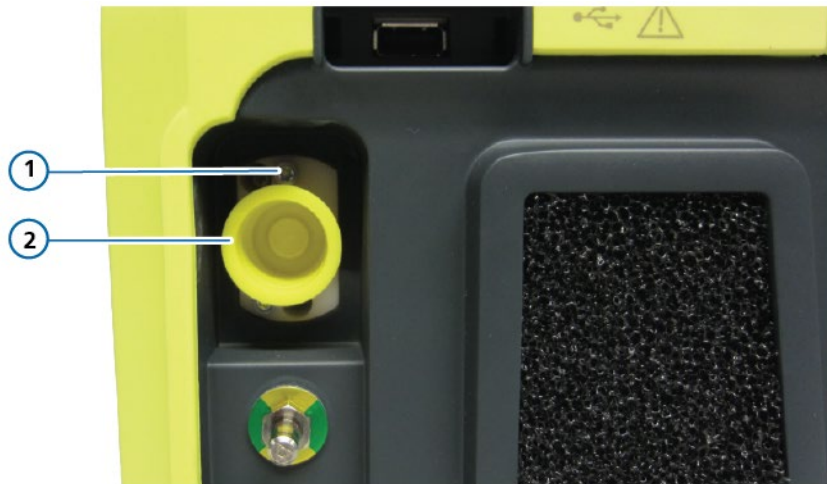
Figure 7-1. Removing the yellow protective cap and screws from the high-pressure oxygen inlet
