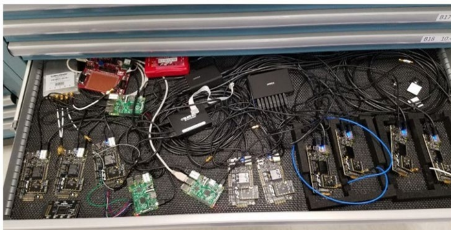
Figure 3-1 Wired RF devices in drawer with splitter and coax cable connectivity
