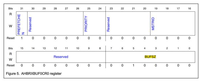
FlexSPI specifies different buffer size for different master. That means some masters may have the dedicated prefetch buffer, which can optimize performance in some applications. The AHB RX buffer is assigned to different masters according to the register fields, AHBRXBUFOCRO [MSTRID] - AHBRXBUF3CRO [MSTRID].
