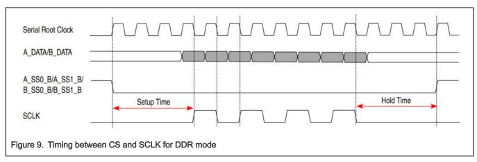
HyperRAM is the device using HyperBus interface and HyperBus interface supports DDR mode. Figure 9 shows the configuration of delay between CS and SCLK. APS6404L PSRAM supports SDR mode, while APS12808L PSRAM supports DDR mode.
