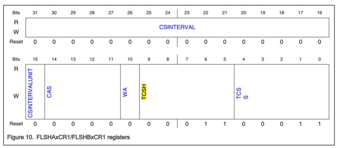
For example, for HyperRAM device, TCSH and TCSS is equivalent to the  $t_{CSH}$  and  $t_{CSS}$  timing parameters. For example, Table 2 shows the related parameters in 7KS0642GAHI02 HyperRAM device.
