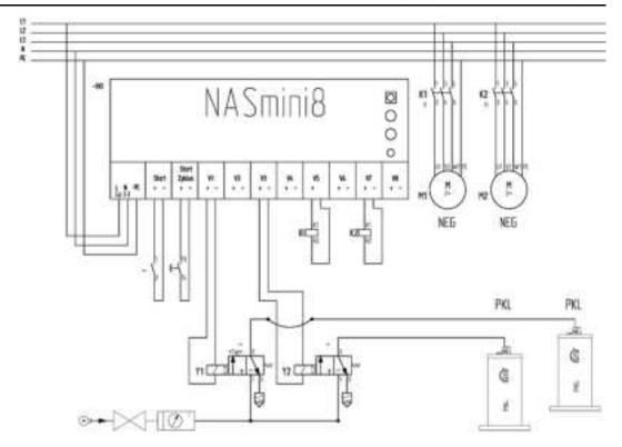
NEG = Electric External Vibrator PKL = Pneumatic Impactor
