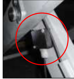
Picture 17 (lower limit switch)
