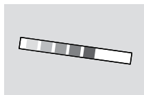
Water hardness test strips
