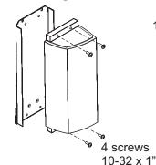
1. Attach the Bose® amplifier to the back side of the C-1332 Hinged Mounting Plate.
