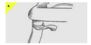
Insert end of flexible cable housing into lever until the housing is completely seated and run housing along handlebar, securing with tape.
