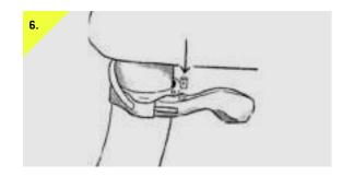
Insert barrel nut into the round floating center blade of the lever. It is crucial that the barrel nut is placed into the curved portion of the floating center blade. Note: The barrel nut that will be inserted into the lever has a hole for the cable to slide through and is tightened using a 2mm and 3mm allen wrench.
