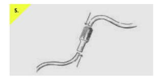
Insert cable originating at dropper post through rotary ferrule and through the housing to the lever.
