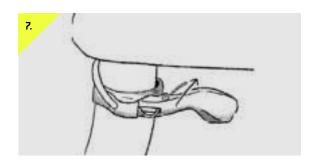
Pull the cable through the lever and hole in the barrel nut until the cable is tight.
