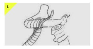
Remove bar tape to expose bare handlebar and cable housing / wiring for proper clamp placement.
