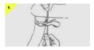
Tighten the barrel nut with a 2mm allen wrench on one side and a 3mm allen wrench on the other side. Note: You may have to back off the 2mm side to open the hole in the barrel nut.
