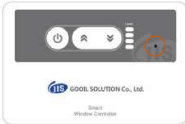
Press the pairing button using a thin tool on the front of the controller.
