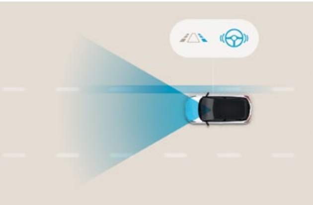
Forward Collision-Avoidance Assist (FCA). Stops your car fast, even if you're distracted. FCA alerts you to slowing or stopped vehicles as well as cyclists and pedestrians in your path – and automatically applies full braking power if you don't react in time.
