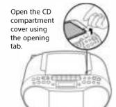
**2** Insert the tip of your finger into the opening tab to open the CD compartment cover.
