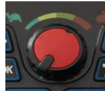
Figure 8 – Max Speed Limiter
