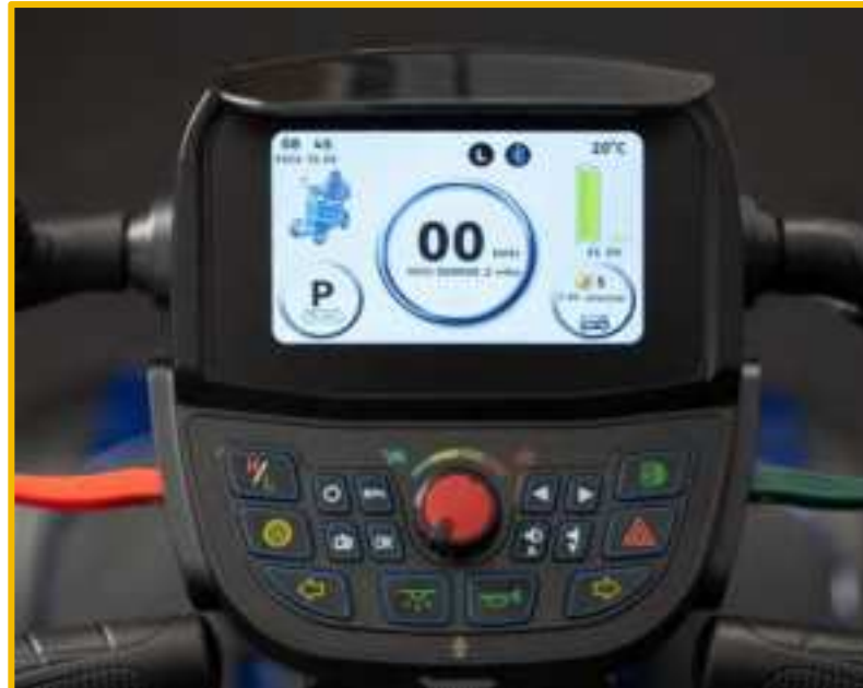
Figure 10 – Digital dashboard displaying data
