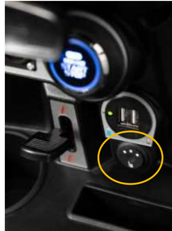
Figure 20 – Heated seat button
