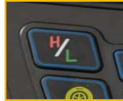
Figure 7 – H/L Speed Mode Control
