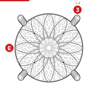
Screw four part 3 fasteners into the part E tabletop.
