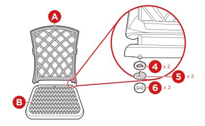
Insert the part A backrest into the part B seat and secure it with two part 4 washers, two part 5 spring washers, and two part 6 nuts.
