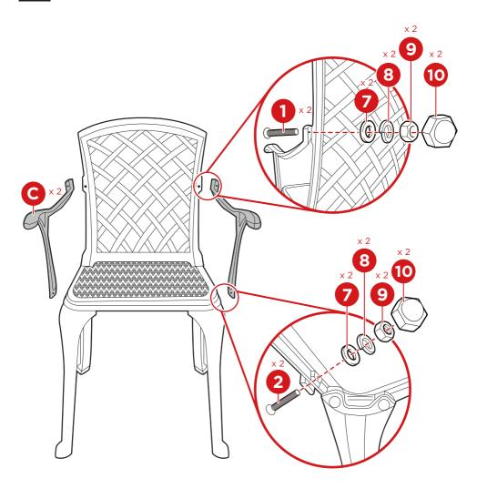
Attach the bottom of the armrest with a part 2 bolt, part 7 washer, part 8 spring washer, part 9 nut, and part 10 nut cap. Repeat to attach the other armrest.
