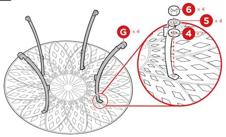
Attach four part G table legs to the fasteners with four part 4 washers, four part 5 spring washers, and four part 6 nuts.
