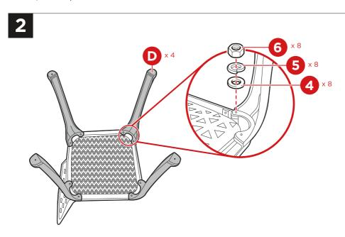
Attach four part D chair legs with eight part 4 washers, eight part 5 spring washers, and eight part 6 nuts – two washers, spring washers, and nuts per leg.
