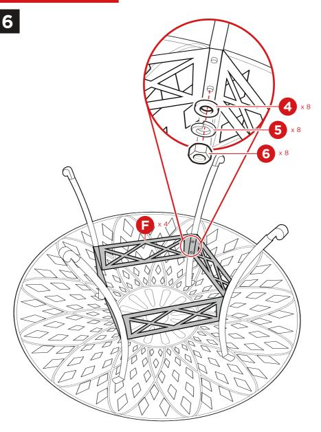
Attach four part F supports to the table legs with eight part 4 washers, eight part 5 spring washers, and eight part 6 nuts.
