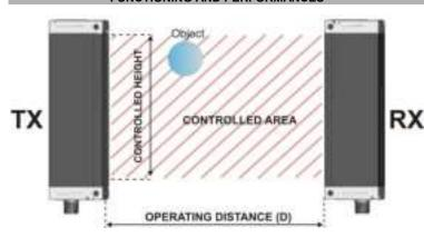
The beam interruption due to the passage of an object inside the controlled area caused the closing of the switching output and the variation of the device analogue output signal. Small objects can be detected (reaching dimensions of only 5 mm) and determine linear measurements with a  $\pm 3$  mm error in best cases.
