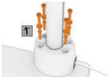
**14** Using the grease packet included in the transducer replacement kit, apply grease to the 4.75 mm ( $^{3}/_{16}$  in.) O-ring on each bolt.
