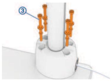
When replacing the transducer, you should dispose of these screws, washers and O-rings. New parts are included with the transducer replacement kit.
