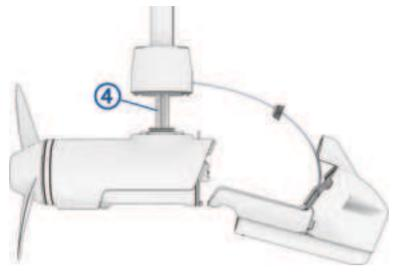
4 Holding the cables only, slowly pull them out of the shaft, taking care that the cable connectors do not get caught on the top of the shaft.
