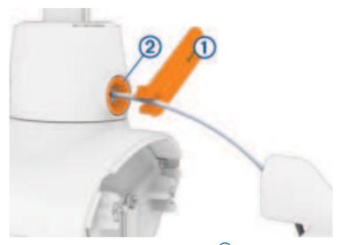
2 Using a ball-head 4 mm hex bit or wrench, remove the screws 3 that secure the shaft base to the propeller drive motor.
