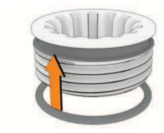
4 With the O-ring facing the transducer, feed the replacement transducer cable through the recessed nut and the hole in the front of the shaft base ①, but do not feed the cable up through the shaft.
