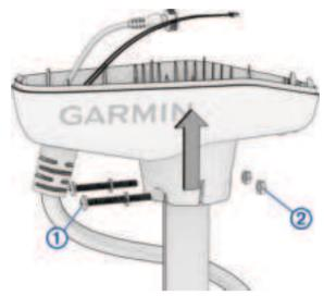
You should keep these bolts and nuts in a safe place, because you must use them when reinstalling the shaft cap.
