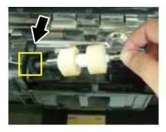
7. Insert the right end of the new Reverse Roller to its slot. If successful, a crispy snap-in sound can be heard.
