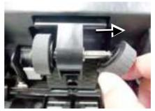
3. Press down the hook next to the left roller to remove the left roller.
