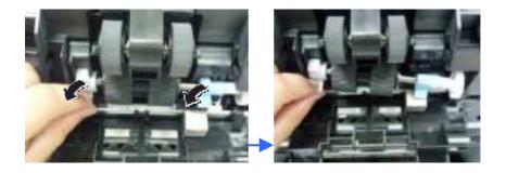
4. Remove the rollers from the shaft.
