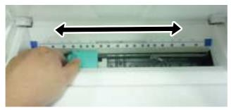
8. Align the arrow mark on the print cartridge holder with the arrow mark on the product as illustrated.
