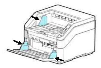
4. Load the stack of document facing up with the top of the pages pointing into the feeder.
