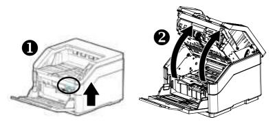
2. Carefully pull the paper out of the ADF unit.
