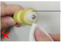
Do not let the cloth moisturized with alcohol touch the foam beneath the surface of the roller or let the excessive alcohol flow into the foam.
