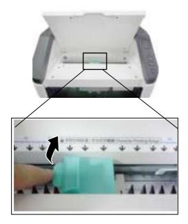
5. Grasp the tab of the cartridge and insert the cartridge into the holder with the label facing up and the tab pointing to the left.
