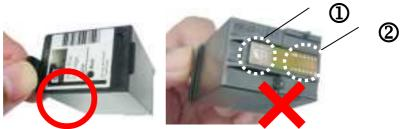
6. Grasp the tab of the cartridge and insert the cartridge into the holder with the print side face up and the tab pointing to the left.
