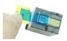
5. Do not touch the ink nozzles (1) or the gold contacts (2) after the tape has been removed.
