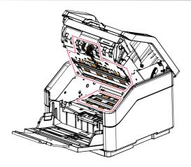
4. Close the ADF by pressing down on the center of the ADF to return it to its original position until it clicks into place.
