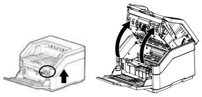
4. Soak a clean cloth with some isopropyl alcohol (95%) and wipe the feeding rollers until they are cleaned.
