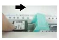
b. Lower the locking lever of the Print Cartridge Holder until it locks in.
