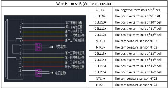
Note: CELL8+ and CELL9- connected with the positive terminal of 8<sup>th</sup> cell and negative terminal of 9<sup>th</sup> cell to provide sampling accuracy of cell. And CELL16+ is also the positive terminals of battery pack.
