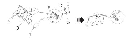
STEP 3 Assemble door (6) and door handle (4) with washer F and screw nut D. Then put on the retainer (5) and fix it with screw nut E.
