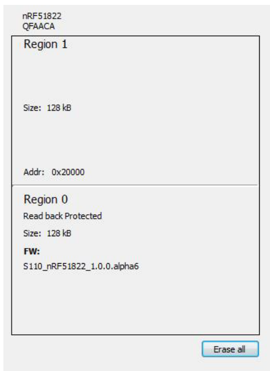
Figure 22 Flash memory organized in two regions with the BTLE stack located a Region 0 and with read back protection on region 0
