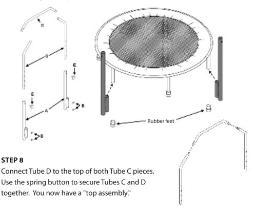
Lower the top assembly into both Tube A pieces until the bottom hole in the top assembly lines up with the hole at the top of each Tube A. You may need to rotate each Tube A for the top assembly to fit. Secure the top assembly in place with the F knob.
