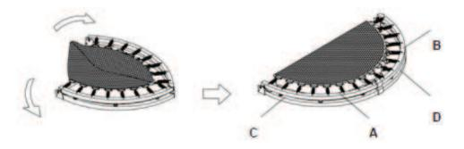
Remove the bracket pin from both ends of the trampoline and place them aside.
