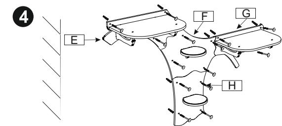
**EN** Install from the bottom up. Install part H first. Use a level to make sure this part is installed evenly. Then install parts F, G, E in stages.
