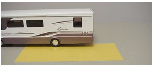
Weighing Left Rear 'Corner'
