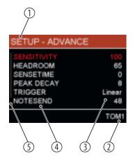
In the 'ADVANCE' submenu, further physical settings for the drum pads can be made. The respective parameters are displayed depending on the trigger.
