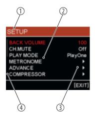
Various device settings can be customised in the Setup menu. The parameters set here affect the entire drum module and cannot be changed by changing the drum kit.
