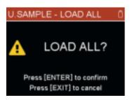
Press [ENTER] to load all files to the USB storage medium. The files are loaded until the maximum number is reached or the storage capacity is exhausted. Press [EXIT] to cancel.
