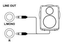
Connect the inputs of your amplifier or active monitor to the output sockets [LINE OUT] on the rear panel of the drum module. Connect a CD or MP3 player etc. to the [LINE IN] input socket on the rear panel of the drum module.
