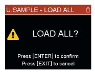
Press [ENTER] to load all files to the USB storage medium. The files are loaded until the maximum number is reached or the storage capacity is exhausted. Press [EXIT] to cancel.
