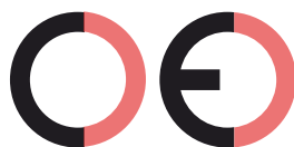
False CE Mark (too far)
