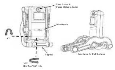
As illustrated above, the BearTrap® body can rotate and be oriented in a variety of ways. Additionally, the body can be rotated through the clamp mechanism for other mounting options. Simply pull the clamp open and rotate the body through the opening. The wire handle may need to be moved to allow full range of motion of the body.
