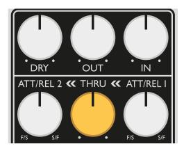
**IN:** This control sets the level into the first compression stage. Higher settings result in more compression, as more signal is pushed over the fixed threshold. The LED on the right will indicate when the first stage is compressing. Increasing the IN control will also make the signal louder, so this should be balanced with the THRU and OUT controls.
