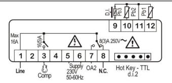
Power Supply (terminals 5-6): 110 or 230 Vac @50 or 60Hz
