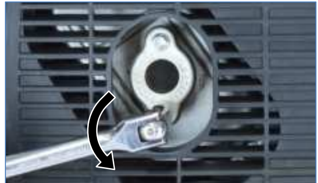
Figure 32 Remove the Spark Arrestor Clamp
