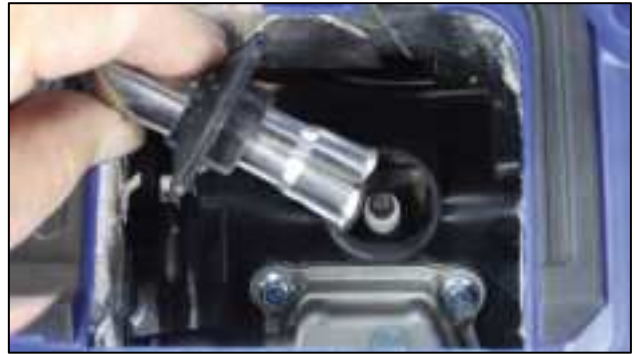
Figure 29 Remove the Spark Plug Boot
