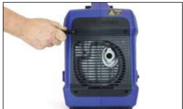
Figure 16 Remove the Muffler Access Cover
