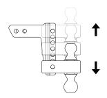
**STEP 1:** Place the Drop Hitch at the desired drop on the drawbar in order to ensure that your vehicle and trailer are properly positioned.
