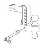
**STEP 2:** Insert the keylock pin into the Drop Hitch when you have achieved the desired position along the drawbar.
