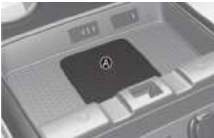
[A] Vehicle authentication pad (Wireless charging pad)
