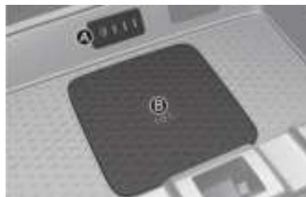
[A] Indicator light [B] Charging pad
