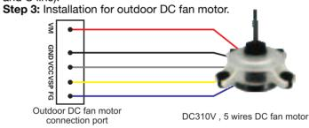
Diagram of DC fan motor connection port: FG(PG) VSP VCC(15V) GND VM(VDC)
