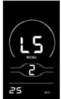
Fig. 5 Speed limit setting interface
