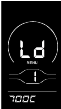
Fig. 4 Wheel diameter setting interface
