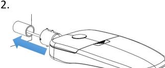
Feed the mains cable into the column and offer the spigot up to the column.
