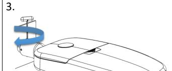
Using the 4mm Allen Key, tighten all the grub screws slightly so the fitting can still rotate.
