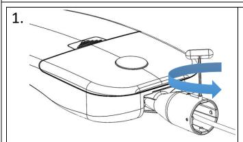
Using a 4mm Allen Key, loosen all the grub screws sufficiently to allow for the column diameter.
