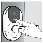
Press the "TOUCH" key, keypad lights up and then press \*\*\*#. While a long beep sound and blue light will blink 5 times for successful removed all user credentials.
