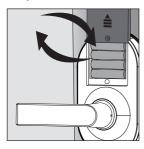
Either when using credentials / passcode / mobile App to unlock or lock the door, or when using the programming card for enrollment, if there is 3 short beep sounds and appear 5 times, and blue light blinks 5 times, meaning the battery is low. Please change new battery immediately.
