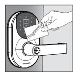
Present the programming card to reading area. Beep sound and blue light blinks in every seconds during process, and 1 long beep / blue light blinks 3 times after 10 seconds means the programming card setup is successful.
