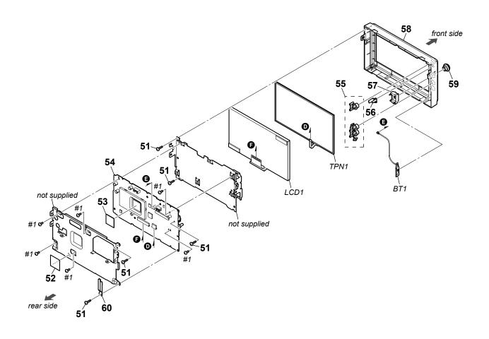
Note 1: Replaced old complete TFT board (Ref. No. 54) is destroyed with the hammer, and throw out it.
