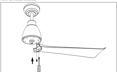
Install the blades to the bottom of the motor. Tighten and secure blade with screw and washer provided. Repeat this procedure until all blades are installed.
