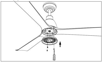
Install the LED light plate onto the steel bracket as illustrated with the 3 supplied screws.
