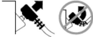
Figure 5-7 Disconnecting Defibrillation Cable from Test Post
