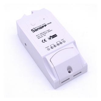
Hi, Welcome to use TH10! Sonoff TH10 can monitor real time temperature and humidity through eWeLink. It supports preset a temperature or humidity range to auto-turn on/off connected device.
