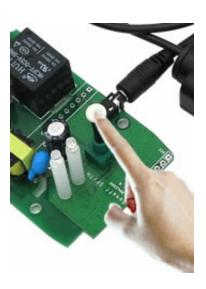
2.Press the button for 7 seconds until the green LED blinks like this: blinks 3 times and on repeatedly.
