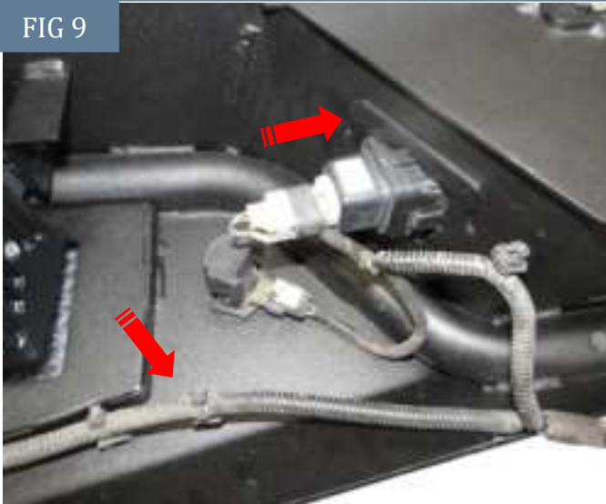
(Fig 9) Attach License Plate lights to mounting slot and wiring harness to Bumper
