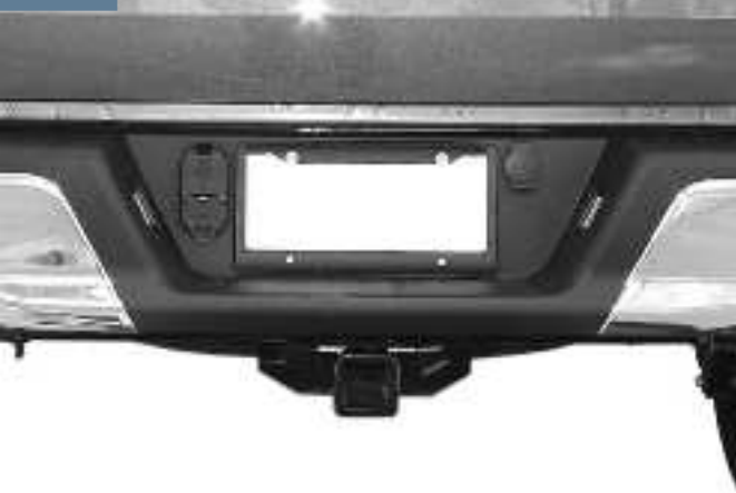
(Fig 1) Unplug and remove 7-wire trailer plug
