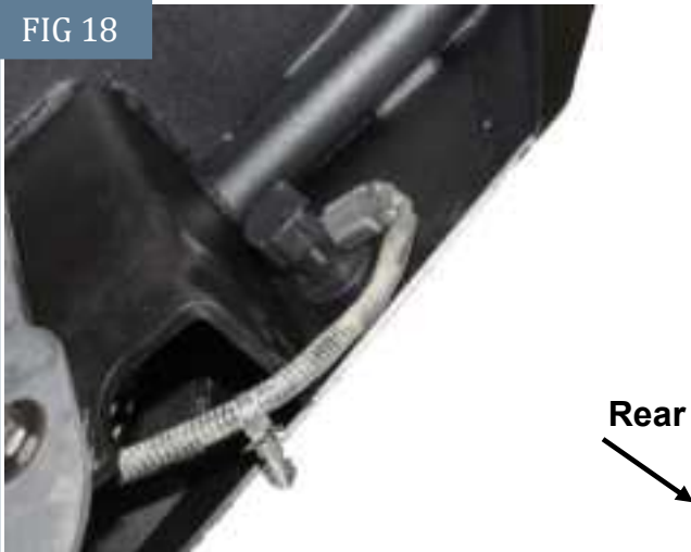
(Fig 18) Attach wire connectors to parking sensors
