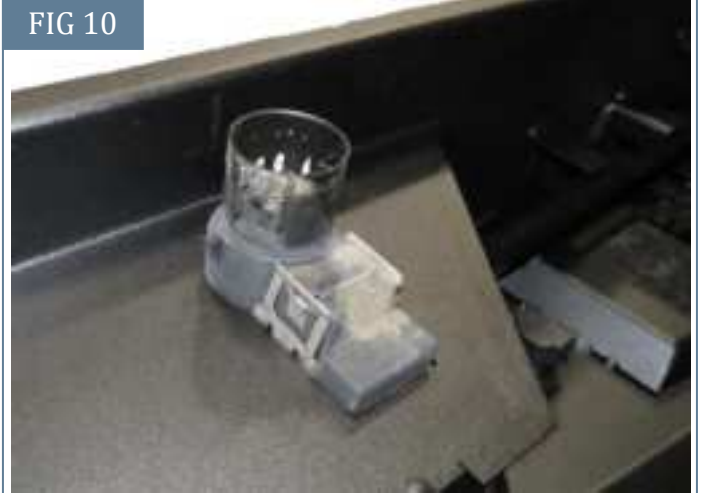
(Fig 10) Attach 7-wire trailer plug to mounting slot
