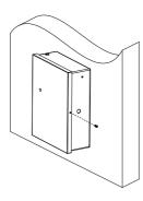
2. Close the case door and tighten the screw on the case door.
