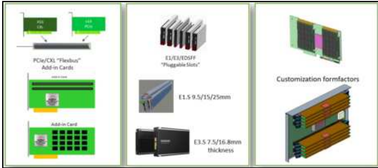
Figure 5. Several CXL memory device form factor implementations
