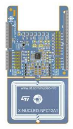
Figure 1. X-NUCLEO-NFC12A1 expansion board
